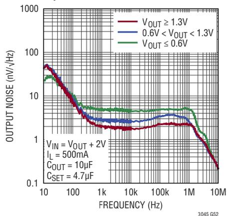
**Output Noise: 10Hz to 100kHz**
