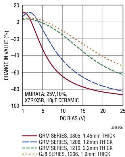
Figure 6. Capacitor Voltage Coefficient for Different Case Sizes
