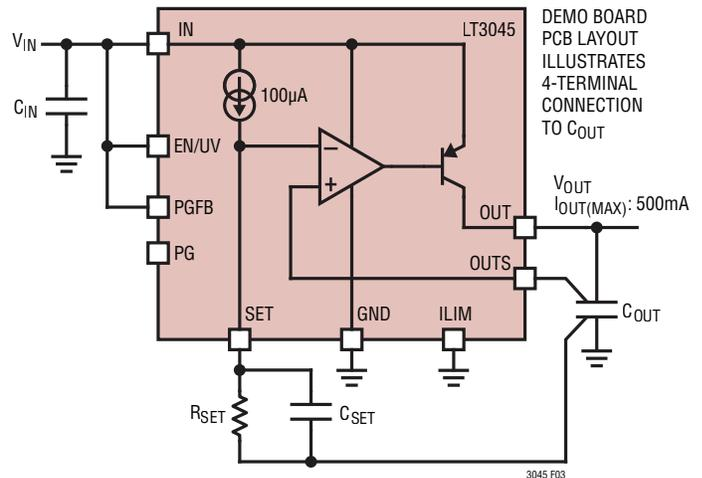
Figure 3. C<sub>OUT</sub> and C<sub>SET</sub> Connections for Best Performance
